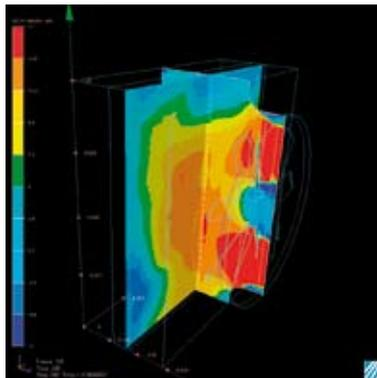
FIGURE 2: A principle sketch of the radiator package on a rock-drill machine and the velocity profile over the radiator surface
