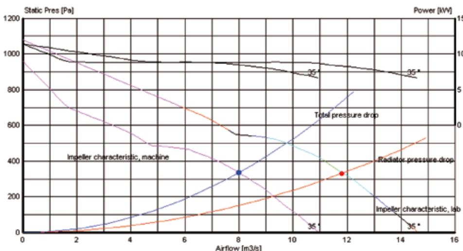
FIGURE 1: The impeller and radiator characteristic showing the difference between ideal laboratory conditions and actual performance of the machine
